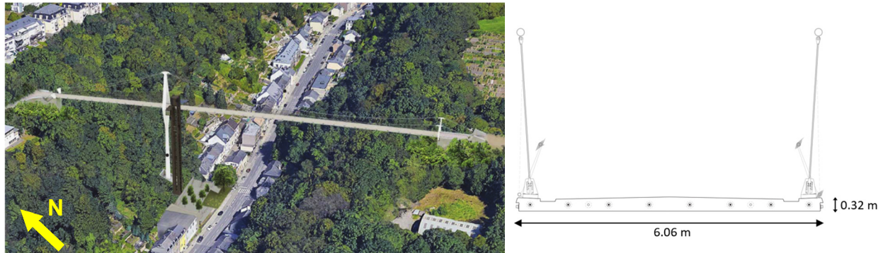
Figure 1. Rendering on the CNW bridge within the Neudorf valley (left) and bridge deck cross-section (right) ( www.vdl.lu ).
